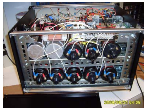
Figure 8. The partially assembled primary ignition system.
