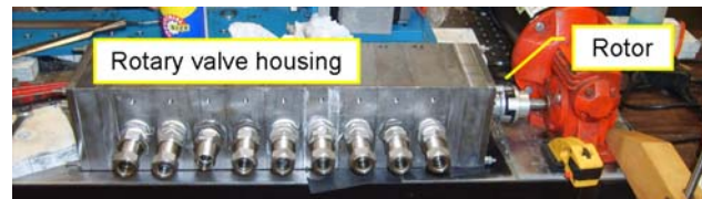
Figure 5. Rotary valve being bench tested.
